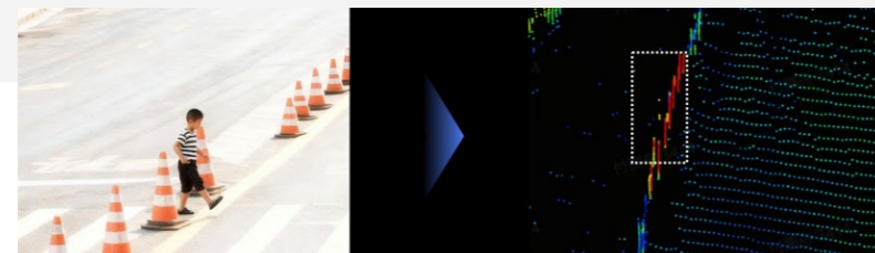
Traditional SPAD solution: Missed detections by erroneous algorithmic filtering
